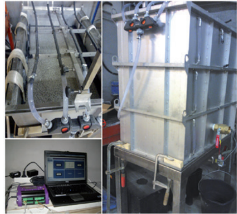
Figure 2. Hydrological simulation of water pervious structures and pavements. Water infiltration capacity, retention capacity, and if needed also water purification capacity, is simulated in a full-scale (adjustable: 330 - 1000 mm) rig, with continuous measurement of the amounts of water: sprinkler irrigation and water passed through the structure.
