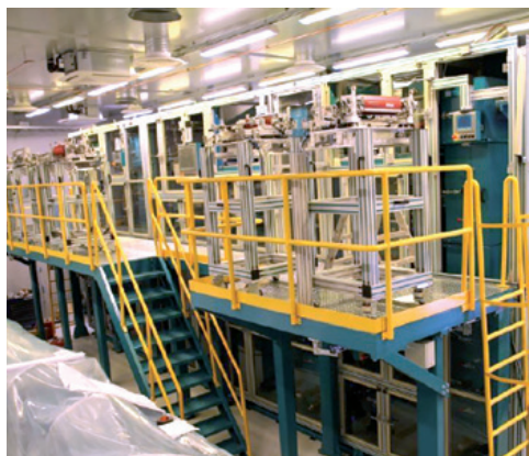
Figure 2. An R2R pilot printing machine
