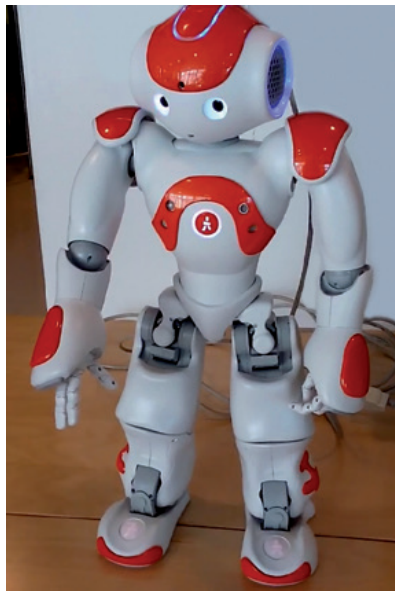
Figure 1. Nao the humanoid robot carrying out reception service tasks. Nao is 57 cm tall so it was put on a table for the comfort of the service users.
