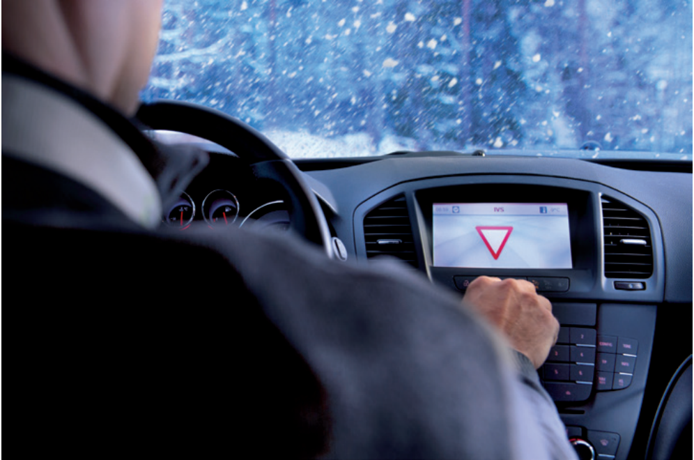
Figure: Cooperative in-vehicle signage function providing information on a give way sign
