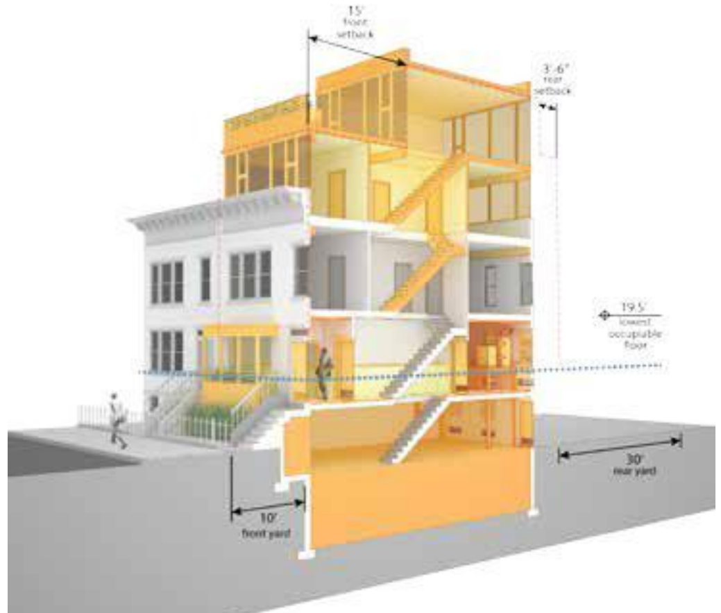
Retrofit strategy for an attached home from Retrofitting Buildings for Flood Risk
